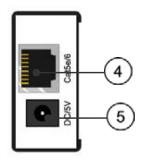
Transmitter HDMI Extender over single Cat5e/6 cable
