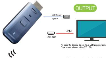
\*Receiver dongle for Output
