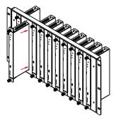
**Step 3:** Use screws to fix mounting ears on the rack to complete the mounting, as shown in the figure below:
