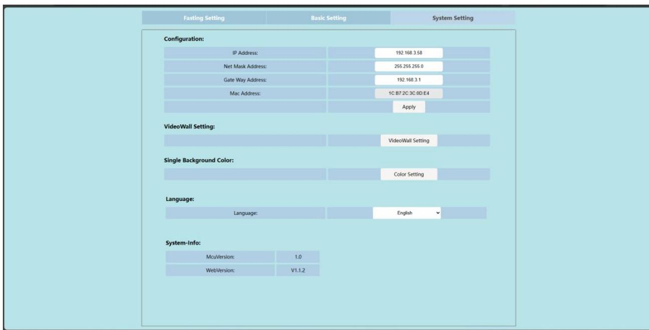
**Configuration:** Set the IP address, gateway address and Mac address etc..
