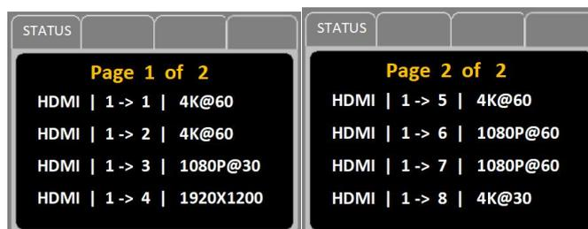
The left column indicates the current audio input format (HDMI supports embedding audio) and the middle part indicates the input and output corresponding status. The right column indicates the current resolution of the corresponding output port.
