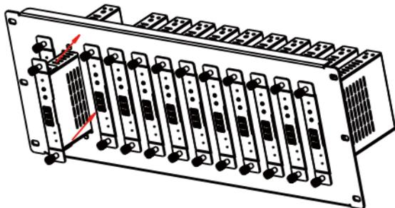
**Step 3:** Use screws to fix mounting ears on the rack to complete the mounting, as shown in the figure below:
