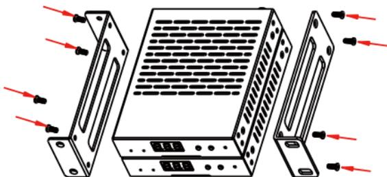
**Step 2:** Fix two 1U rack panels on another two stacked products in the same way, then use screws to fix two 1U rack panels together, as shown in the figure below:
