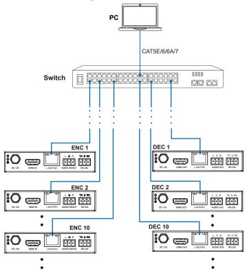
**Step 2:** Set the PC's IP address to be in the same network segment with the Encoder (default IP address: 169.254.100.254)/Decoder (default IP address: 169.254.100.253), for instance, set the IP address to be 169.254.3.150 and Subnet mask to be 255.255.0.0.
