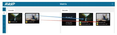
② Left-click the Encoder and drag it to All Decoders, then release the mouse to realize one-to-all switching.
