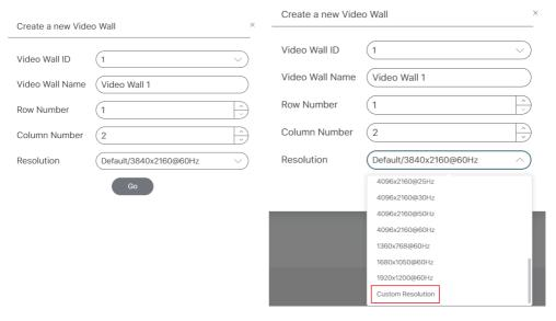
You can set the Video Wall ID, Video Wall Name, Row Number, Column Number and Resolution. Then click "Go" to create the video wall. If the "Custom Resolution" is selected as the resolution, more detailed customizations can be set, as shown in the following figure.
