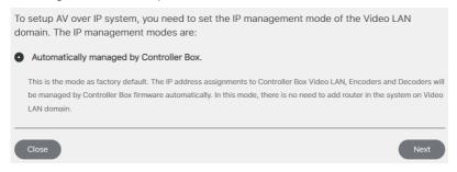
**Step 3:** Select "Automatically managed by Controller Box" as the IP mode of Video LAN. The IP addresses of the Video LAN port, Encoder and Decoder will be assigned by the Controller automatically, and the connection method is as following.
