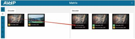
③ Left-click the Encoder and drag it to multiple Decoders, then release the mouse to realize one-to-many switching.
