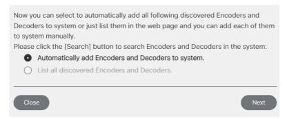
Select "Automatically add Encoders and Decoders to system" (Note: The other option is temporarily unavailable), and click the "Next" button to enter the Device page, the system starts to search for devices. All the connected devices will be searched and added into the system (presented in the Encoder/Decoder list) automatically, as shown below.
