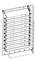
**Step 3:** Use screws to fix mounting ears on the rack to complete the mounting, as shown in the figure below:
