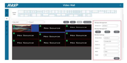
**Step 3:** Select signal source and set the position/size for each window as required in the same way. Then, click "Apply" above the video wall canvas to save the current settings as Preset 1 and take effect, as shown in the figures below.
